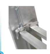
**d) Rope-operated ladder assembly** There is a danger of injury when extending the upper section of ladder. As the control device on the stile slides along the lower section of ladder, the ladder should only be held by the rungs of the extension and by the rope.
